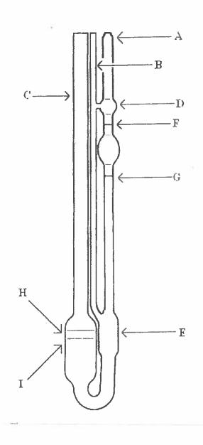
Figure 1. Ubbelohde Viscometer
